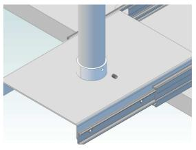
Thread the support pole into the female coupler on the top of the slide unit. The pole may not thread all the way into the coupler. Make sure that the pole is threaded far enough in so that the set screw comes in contact with the threaded portion of the pole.
