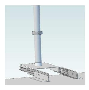
Next attach the "Wall Plate" to the NPT Pipe adaptor with the supplied (6) bolts and nylon lock nuts.
