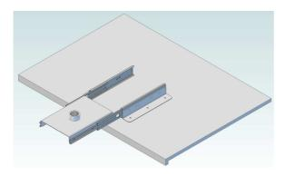
Properly align the slide unit to the desired location on the surface the SL001 is to be mounted on. Using a drill and a ¼" drill bit, drill a hole in each location (6 total) in the Shelf. (Make sure each slide bracket is equal distance from the leading edge of the shelf)
