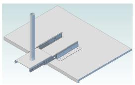
Install the supplied set screw to secure the support pole into place.
