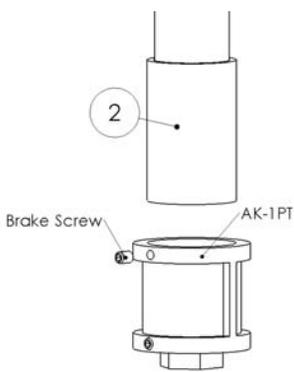
Step 3: Securing the inner mast
