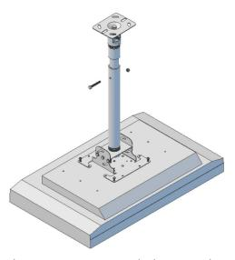
9. There are set screws and a hex wrench provided to secure the mast to the ceiling plate and the mounting head. You will find small threaded holes in the side of the area where the mast threads in. These set screws tighten into the threads on the mast and slightly deform the thread, making it nearly impossible to remove the mast. This is an additional safety feature and you don't want to install these set screws until you are positive you will not need to remove the mast again.
